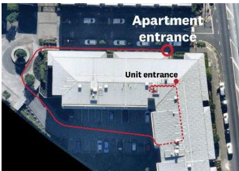
Figure 24: Circuitous step-free route needed to be taken by participant when using mobility assistive devices from their unit entrance to apartment entrance (P8 AP)
