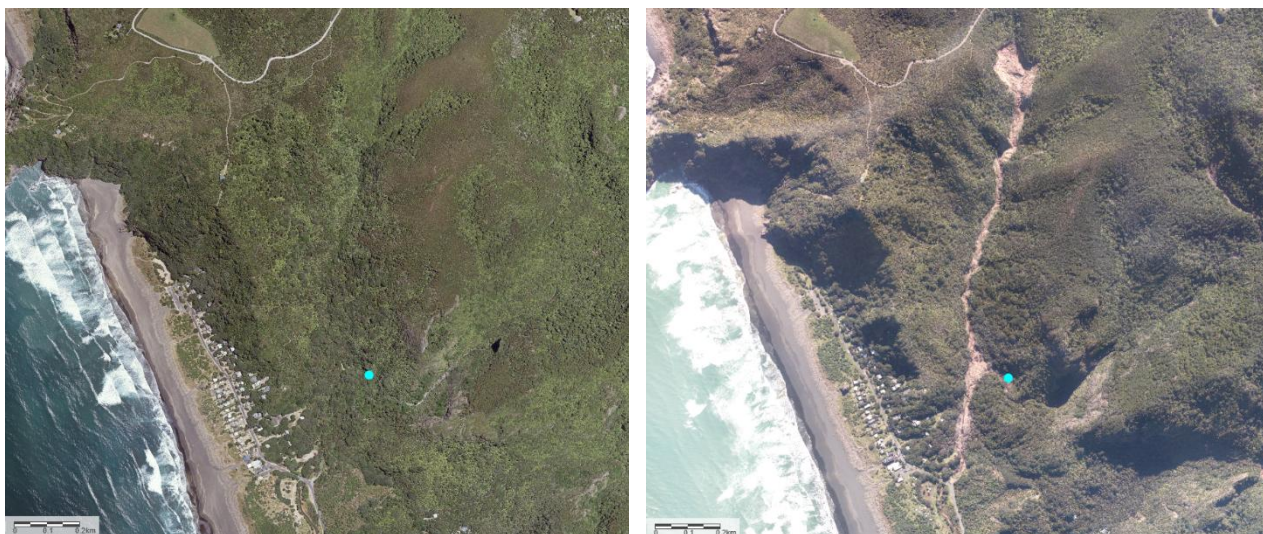
Figure 7-1: Aerial views of Marawhara Stream monitoring site (blue dot) and catchment before and after Auckland Anniversary floods/Cyclone Gabrielle. The image on the left is from 2022 and on the right from 2023, showing the extensive erosion and debris slide affecting the valley (Auckland Council GeoMaps).
