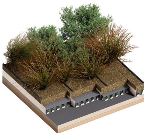
Figure 39: Modular Living Roof Cross-Section and Example
