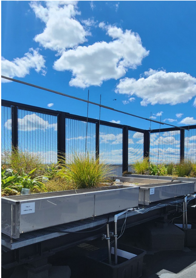
Figure 26: Living Labs, living roof monitoring, University of Auckland Source: The Urbanist
