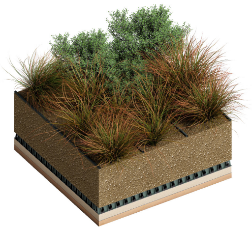
Figure 35: Semi-Intensive Living Roof Cross-Section
