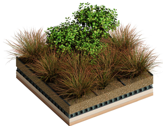
Figure 34: Extensive Living Roof Cross-Section and Example
