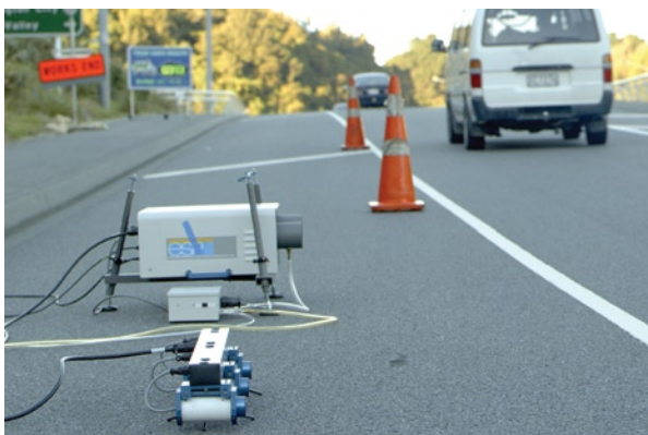
FIGURE 1 On road monitoring equipment and smart sign in the background (Source: NIWA). Emissions are calculated by measuring the changes in (UV and IR) light as it passes through the emissions from a vehicle's tailpipe.
